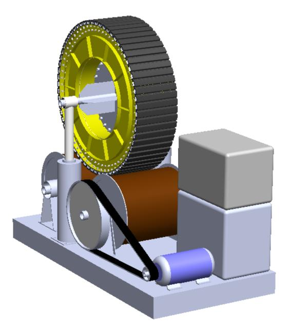
The driving and driven drums are coated with sand-and-gravel bonded in epoxy. The abrasive coating can be rejuvenated and the drums can be replaced with drums coated otherwise.
